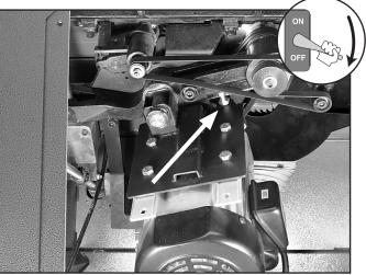
Figure 80. V-belt tension bolt.
